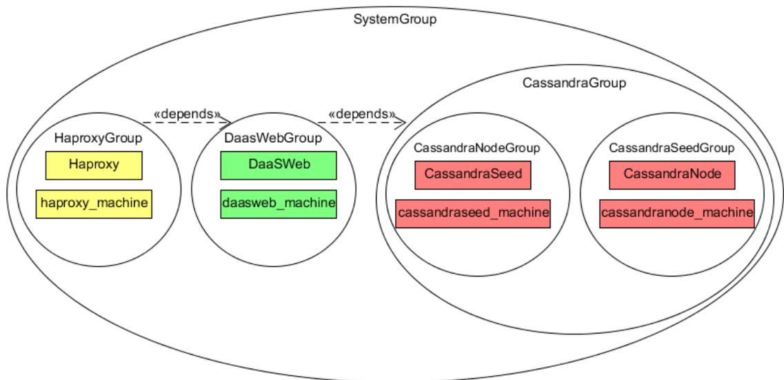
Figure 9: Diagram illustrating the topology defined in Listing 3.9.
