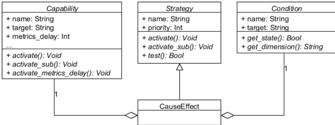
Figure 7: Class diagram illustrating the Capacity, Strategy, and Condition classes. Also included is one concrete Strategy class, CauseEffect.
