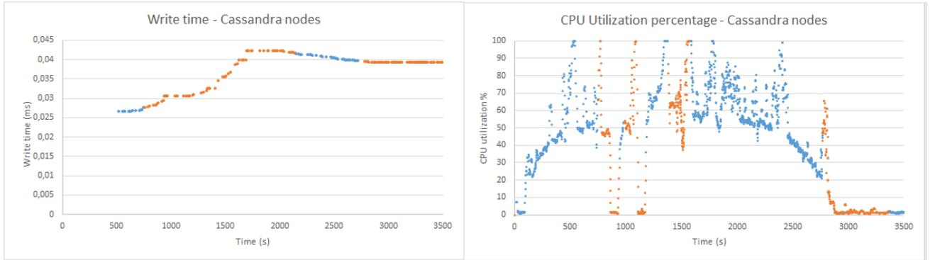
Figure 18: Calculated write time and CPU utilization percentage of the Cassandra node machines during the test period.
