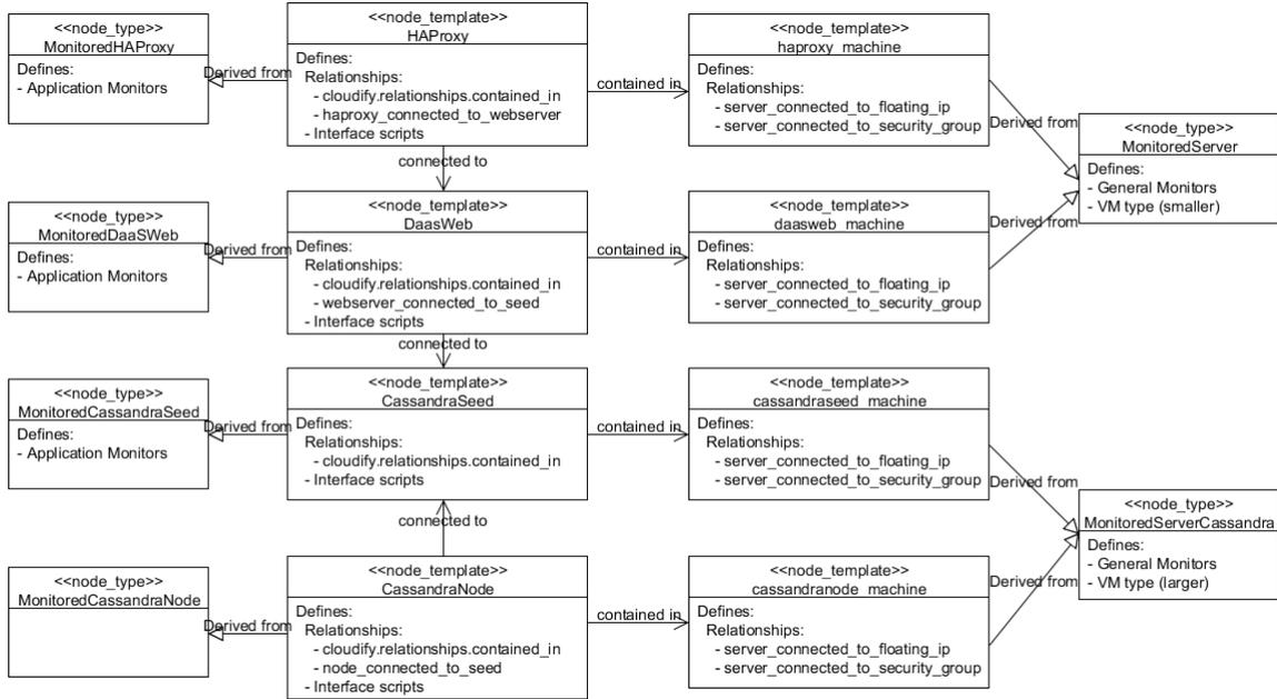
Figure 11: Diagram illustrating nodes and relations in M2M DaaS' Cloudify blueprint.
