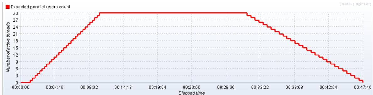
Figure 12: Amount of client threads during the test period. Taken from JMeter.
