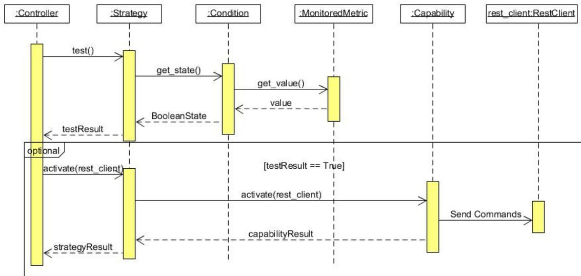
Figure 8: Sequence diagram detailing the test and activation of a strategy.
