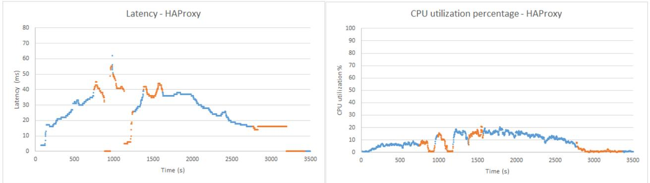
Figure 16: Calculated latency and CPU utilization percentage of the Haproxy during the test period.
