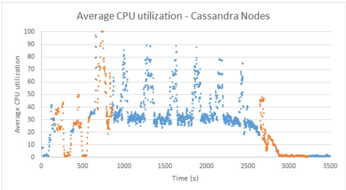
Figure 15: Calculated average CPU utilization percentage of the Cassandra node machines during the test period.
