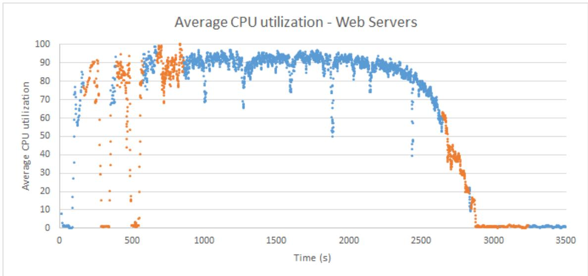
Figure 14: Calculated average CPU utilization percentage of the web server machines during the test period.
