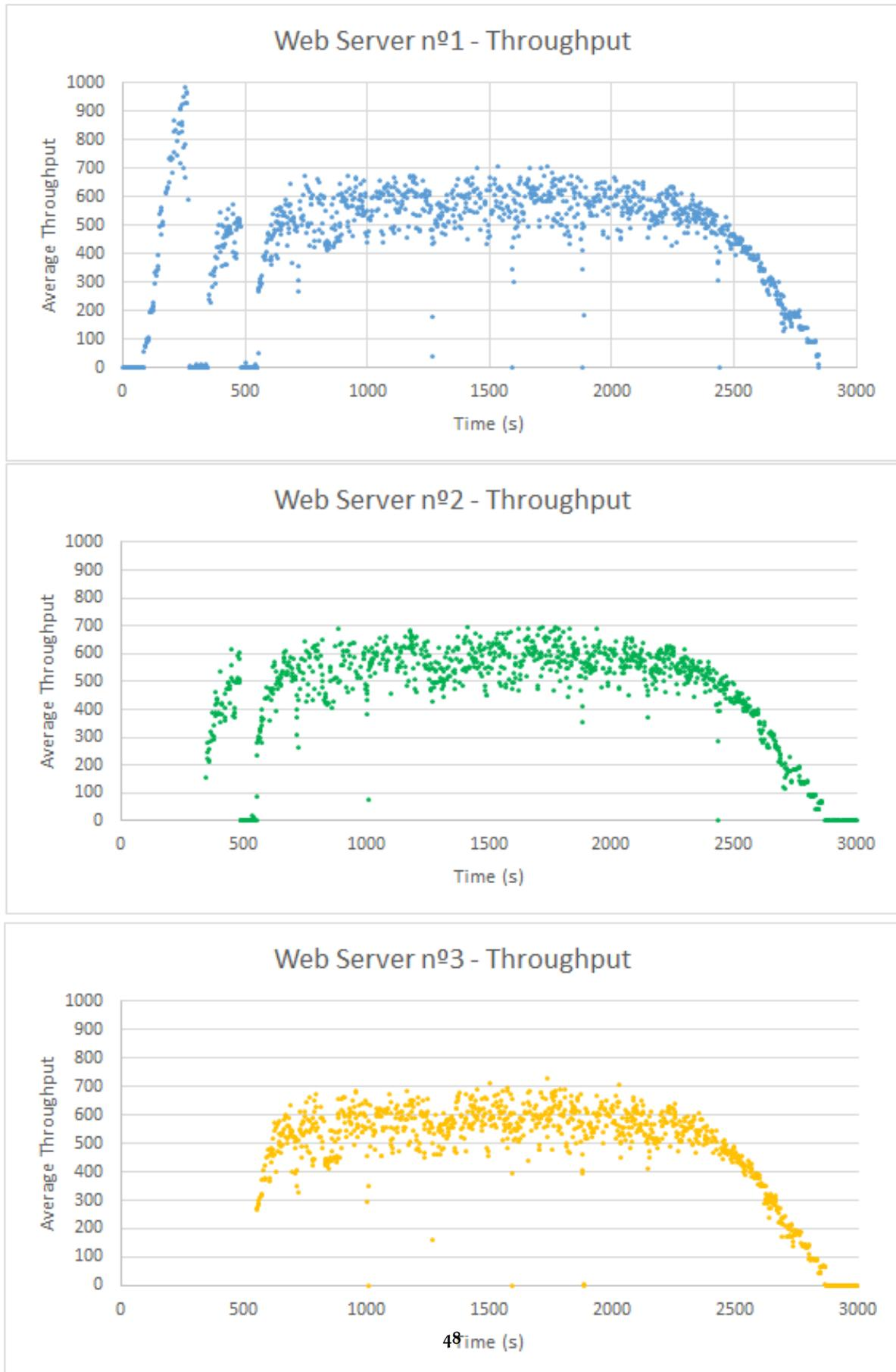
Figure 13: Calculated average throughput for each web server machine during the test period.
