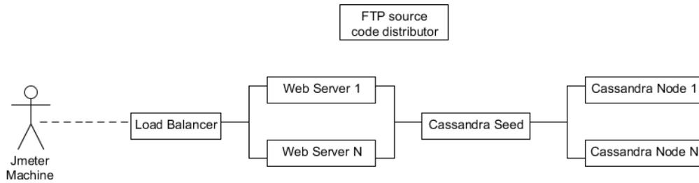
Figure 10: M2M DaaS application topology. Adapted to include a FTP server to provide the application's source code.
