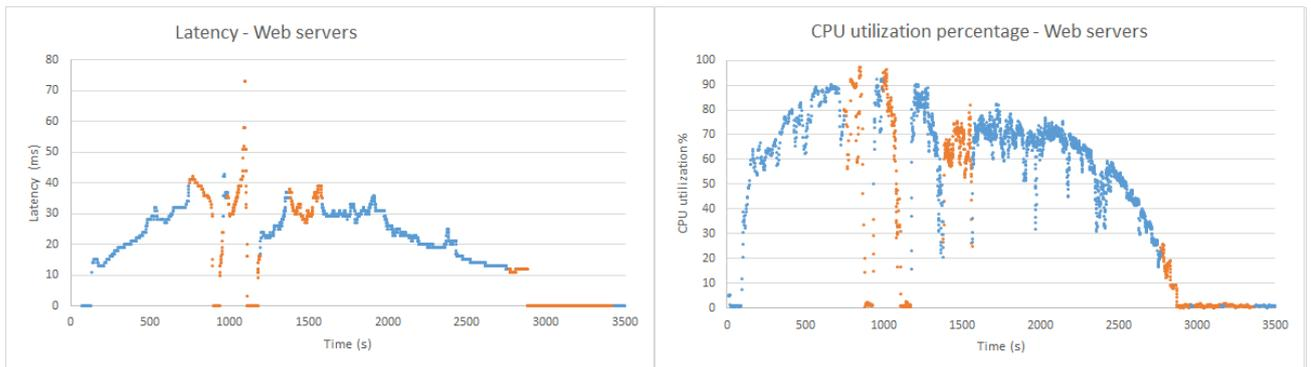
Figure 17: Calculated latency and CPU utilization percentage of the web server machines during the test period.
