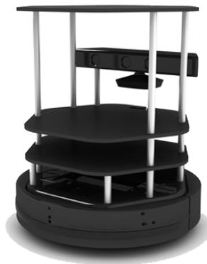
Figure 4.: Turtlebot 2, a robot that uses Kobuki as a mobile base.
